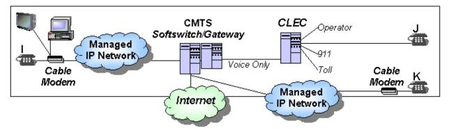
The above example depicts VoIP used in conjunction with a cable TV local network. The example shows how voice services may be delivered to customers using the same fiber and coaxial distribution facilities as are used to deliver data and video services. Customer premises equipment is shown connected to the cable TV company's "head end" facilities whose main components consist of a CMTS (Cable Modem Termination System), "softswitch" and "media gateway".
