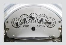
the meter move. The number of revolutions is recorded by the dials that you can see on the face of the meter. The speed of the revolutions depends on the amount of current drawn; the more power consumed at any one instant, the faster the gears will rotate.
