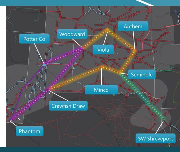
A 765 kV backbone both meets system needs and lays foundation for future regional grid
