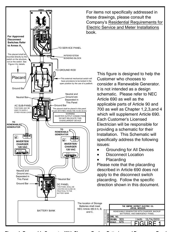
Figure 1: Renewable Generator With Charger, Backup Batteries, and Emergency Panel
