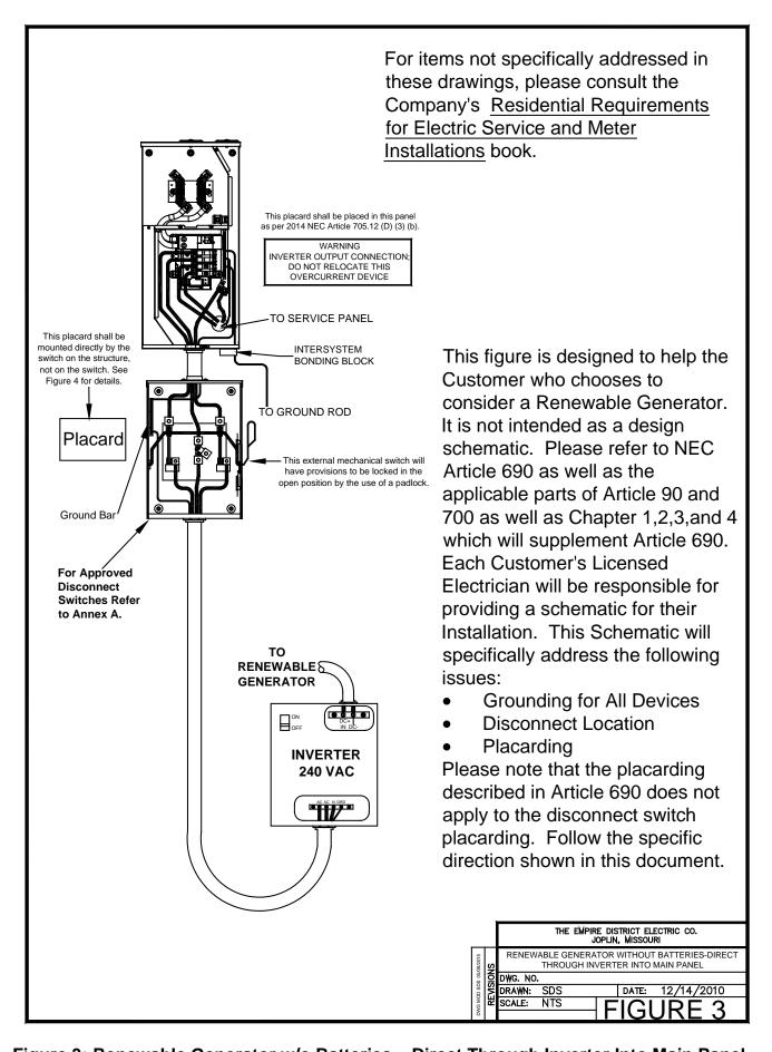
Figure 3: Renewable Generator w/o Batteries – Direct Through Inverter Into Main Panel
